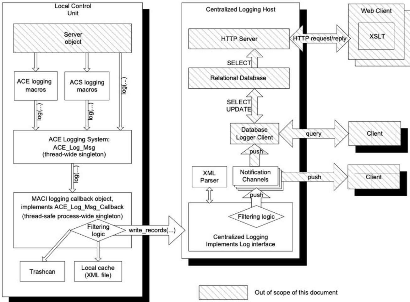
Figure 1: Architecture of the logging system.
