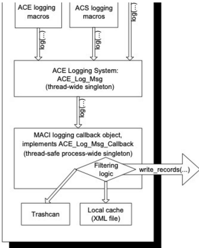
Figure 2: Architecture of the ACE Logging framework.
