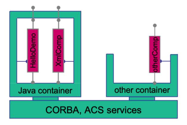
The two Java components, HelloDemo and XmlComponent, can either run collocated inside one Java container as shown, or run in separate Java containers. The Java container is drawn as a closed box to indicate that it works as a "tight container" (cf. [1]), intercepting all functional calls to any of its components, in addition to starting/stopping the components and providing explicit services to them.
